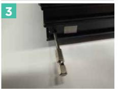
Use a 2.5mm allen key to tighten the joint making sure the top and bottom profile surfaces are level with each other.
